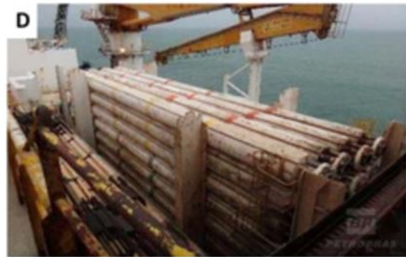
Riser joints on the riser deck of the PSV
